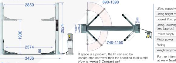
1900 mm/Ad 2050 Lifting height max. Lowest lifting point 96 mm Lifting, lowering 45/30 sec. time (approx.) 230 V Power supply Motor power 2,2 kW Fusing 16 A / type C Weight (approx.) 600 kg Further information to be found
