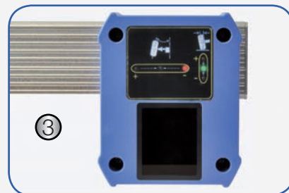
(1) Measuring head with wheel clamps (2) Display on measuring head (3) LED display for Camber and Toe (4) User friendly software with extensive car database
