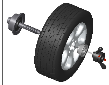
Illustration: Method B - external cone
