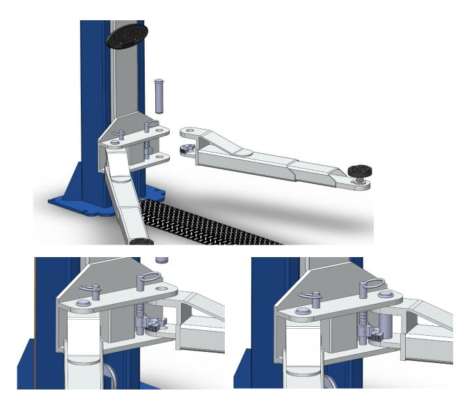
Insert the support arm, lifting the support arm rotation lock. Insert bolt, secure with circlip.
