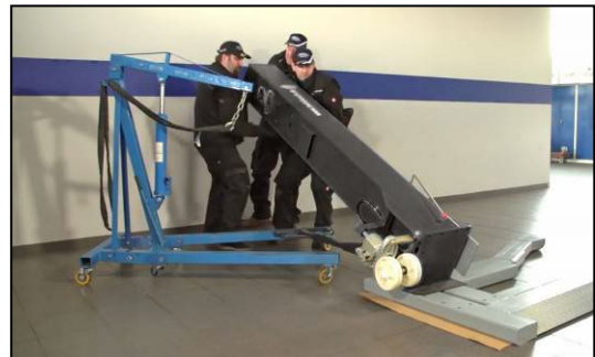
Illustration: Erecting the column
