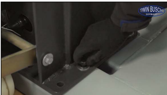
Illustration: Tightening the column
