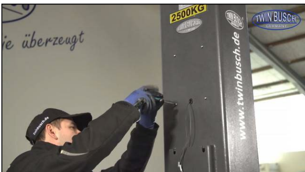
Illustration: Screws mounted on the column
