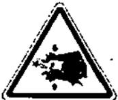
Hand-crushing hazard between turntable jaws.
