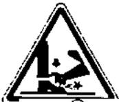
Feet-crushing hazard during turntable turning or operating
